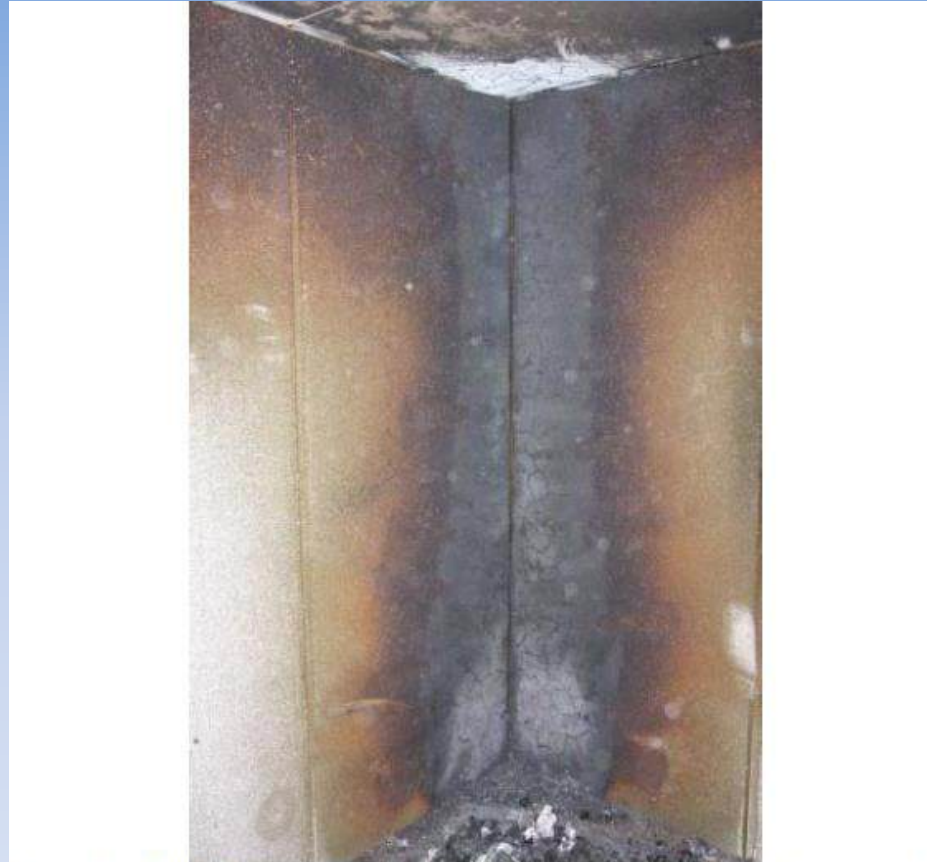
Figure 11. With skin removed charring of foam in region of direct flame contact
